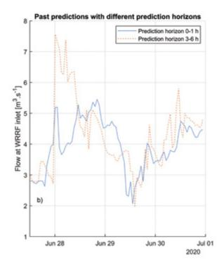
Figure 3.6 (a) Example of model predictions for influent flow to the WRRF using the default control strategy (solid line) and the recommended control strategy suggested by the model (dashed line); (b) Example of past model predictions with different prediction horizons (0-1) hours and (0-1) hours.
