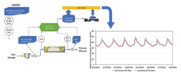
Figure 3.8 Data flow schematic within digital twin for influent load development for the influent "soft sensor"
