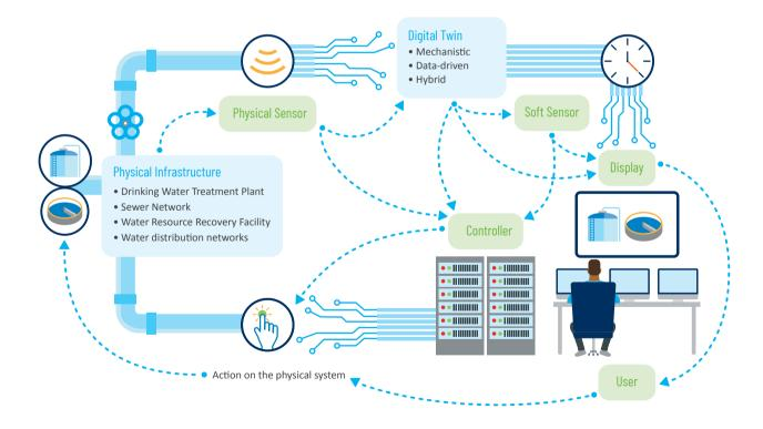
Figure 3.4 Basic structure of a digital twin application. Elements in blue are basic elements needed for implementation of a digital twin, while elements in green are complementary to the digital twin, ultimately to enable an action on the physical system.
