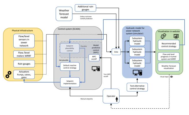
Figure 3.5 Sewer network digital twin structure and components in the current implementation as well as with model predictive control (work is now underway with the goal of implementing full real-time model predictive control).
